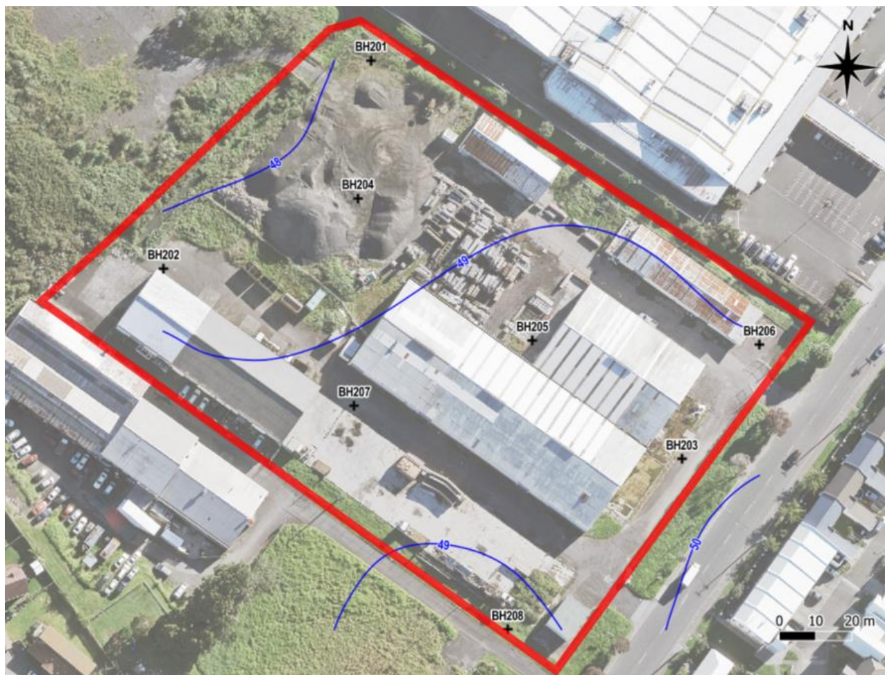
Figure 10: Indicative Groundwater Contour Plot (April 2021 Monitoring Results)
