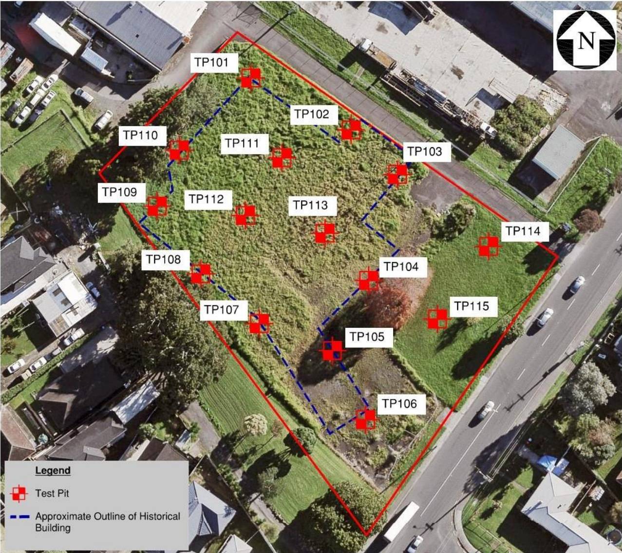
Figure 8: 119 May Road Exploratory Hole Plan. Image Source: AC GeoMaps
