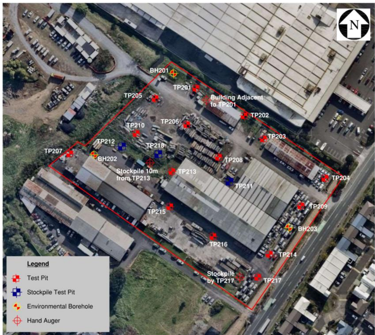
Figure 7: 105A-109A May Road Exploratory Hole Plan. Image Source: NearMap
