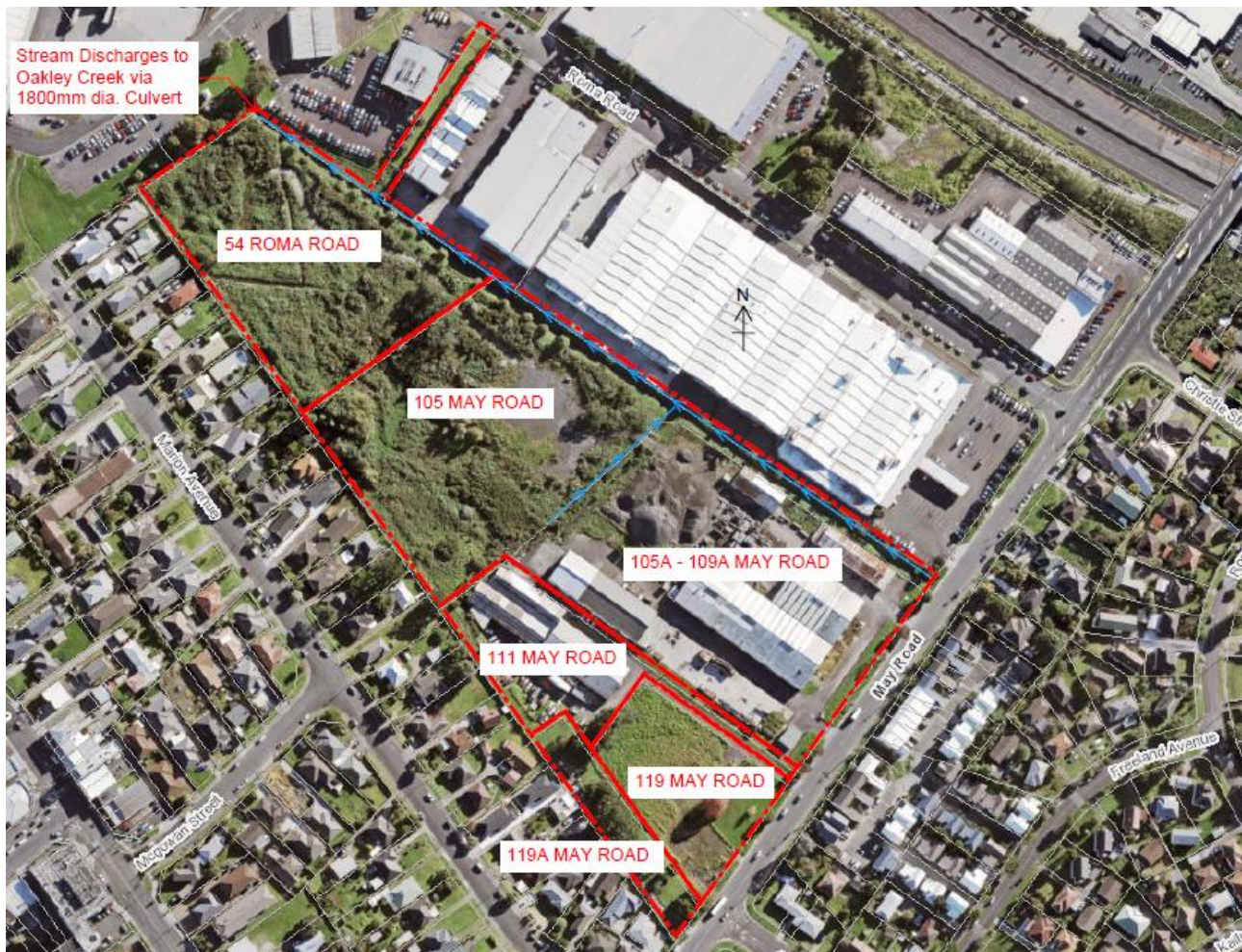
Figure 3: Site Parcels (red) and Main Drainage Channels (dashed blue) (Image Source: Nearmap Australia Pty Ltd)
