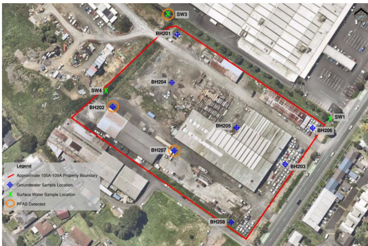
Figure 11: Plan illustrating sample locations with PFAS detections (Image Source: Nearmap Australia Pty Ltd)
