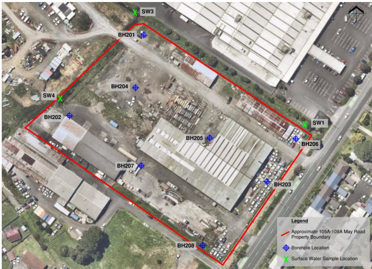
Figure 9: 105A-109A May Road Phase 2 Sample Location Plan (including BH201-BH203 from Phase 1) (Image Source: Nearmap Australia Pty Ltd)
