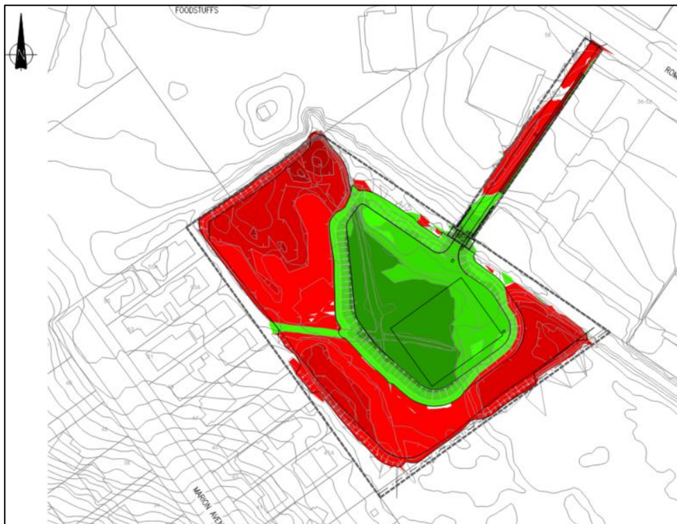
Figure 3. Earthworks Proposed Cut/Fill at 54 Roma Road.
