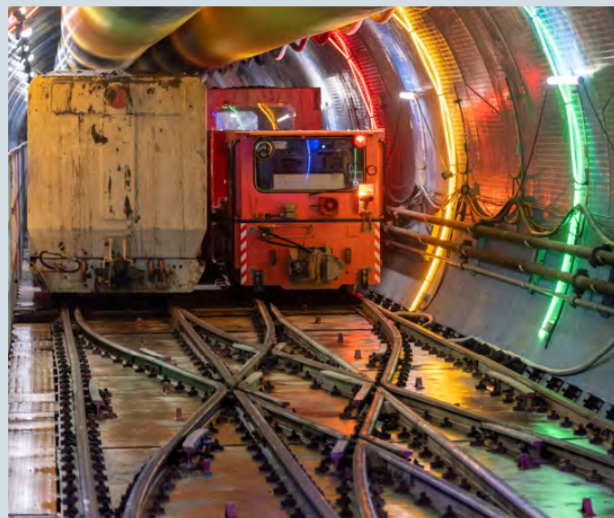
In the main CI tunnel, the electric spoil haulage locomotive is ready for its next trip
