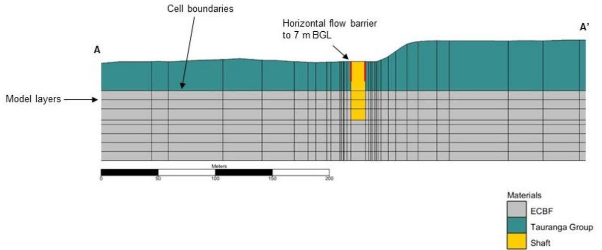
Figure 6. Model grid cross section showing shaft and boundary conditions
