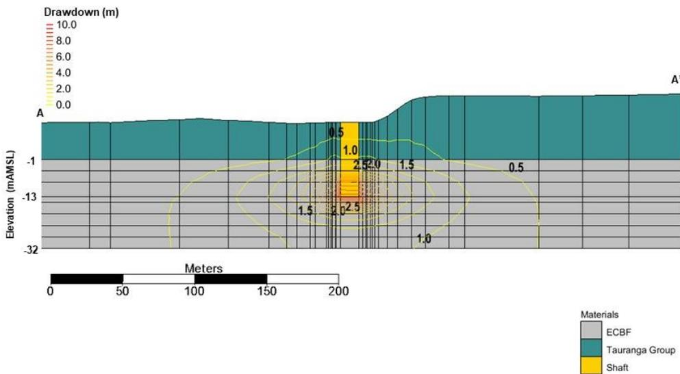
Figure 3. East-west cross-section of predicted drawdown under Scenario 6 conditions.
