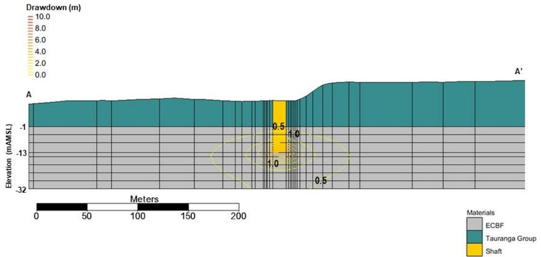
Figure 2. East-west cross-section of predicted drawdown under Scenario 4 conditions.
