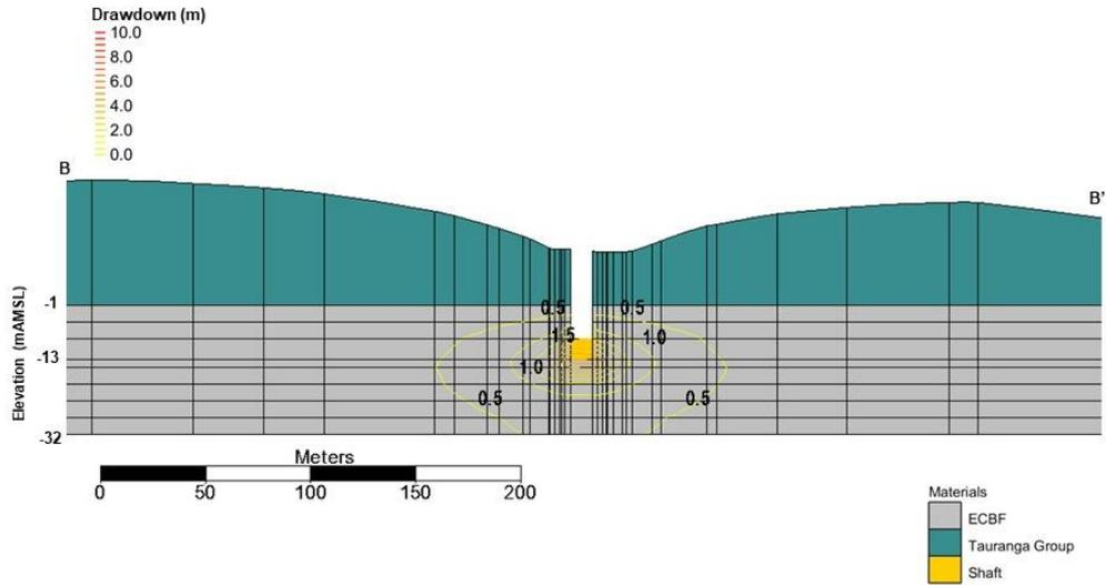
Figure 4. South-north cross-section of predicted drawdown under Scenario 4 conditions.
