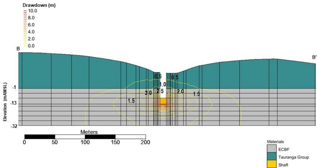
Figure 5. South-north cross-section of predicted drawdown under Scenario 6 conditions.
