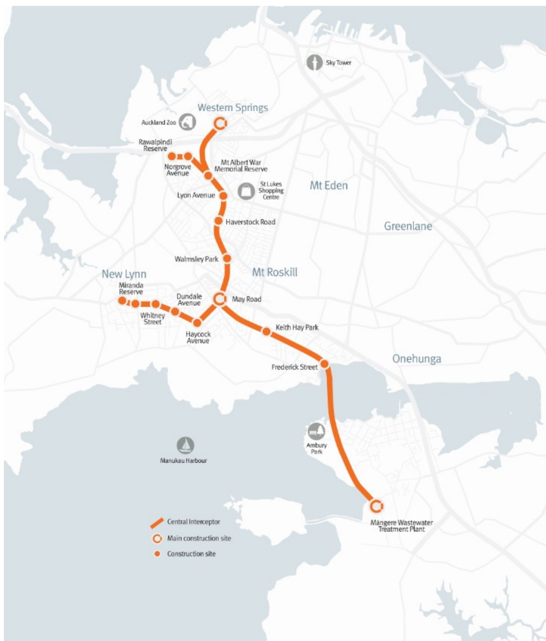
Figure 2: Central Interceptor project alignment and shaft sites
