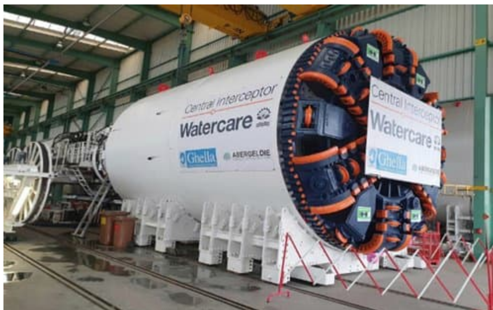
Figure 4.2: TBM at factory testing
