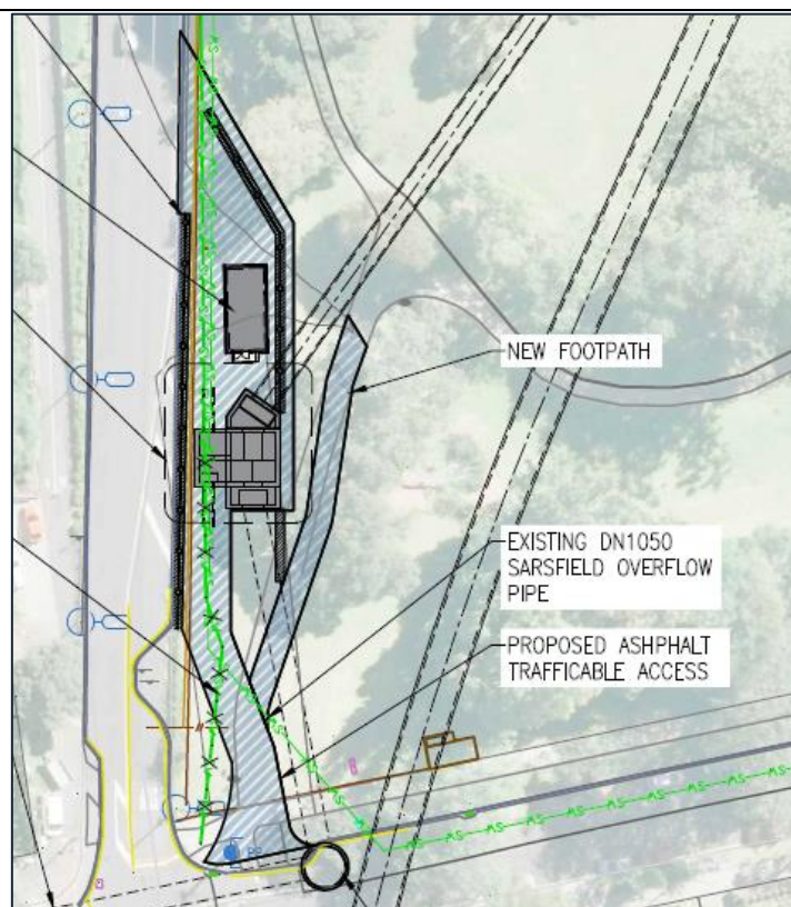
Figure 2: Proposed permanent entry from Sarsfield Street and egress onto Curran Street Site General Layout, Watercare drawing CI-STAT&PLAN, DWG no 2013964.002, issue 2.
