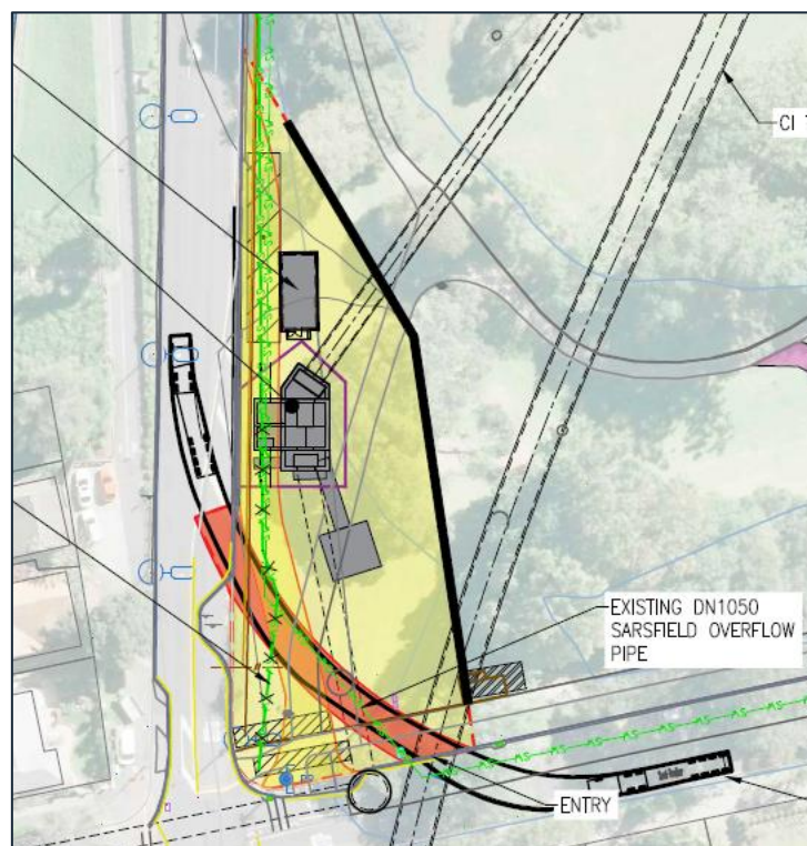
Figure 2: Proposed permanent entry from Sarsfield Street and egress onto Curran Street Site General Layout, Watercare drawing CI-STAT&PLAN, DWG no 2013964.002, issue 2.
