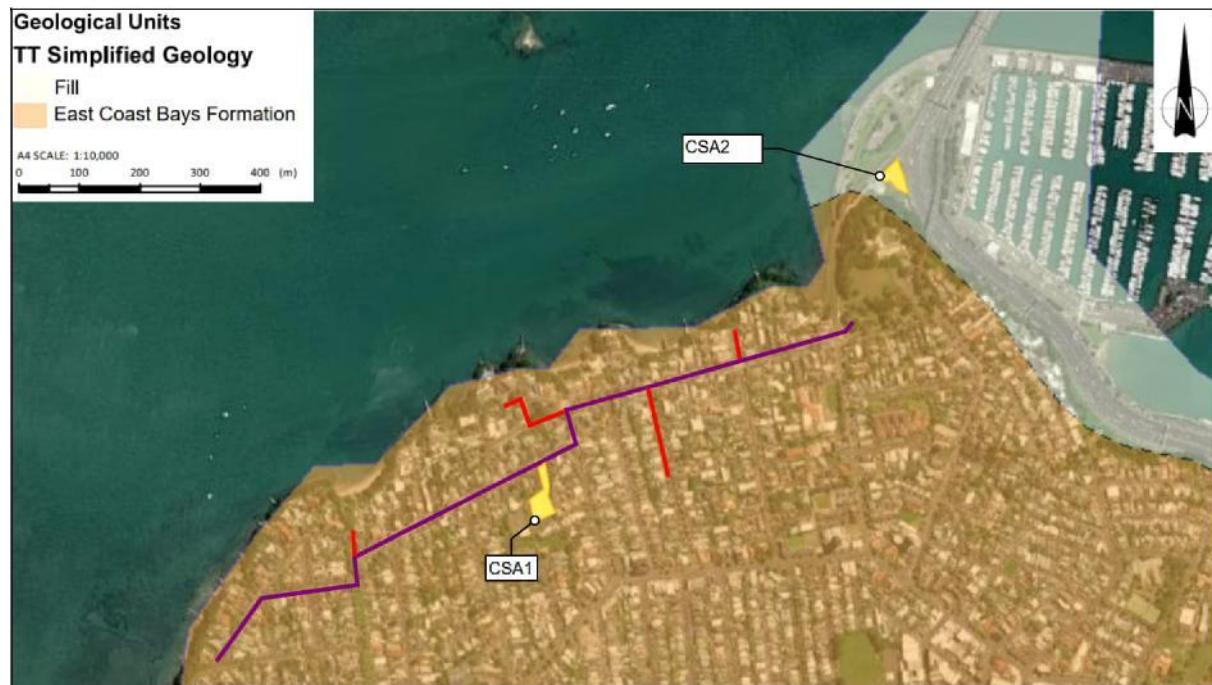
Figure 2.4: Published geology map of alignment, connecting pipes, CSA1 and CSA2 Option 1 and surrounding area (source: Kermode).
