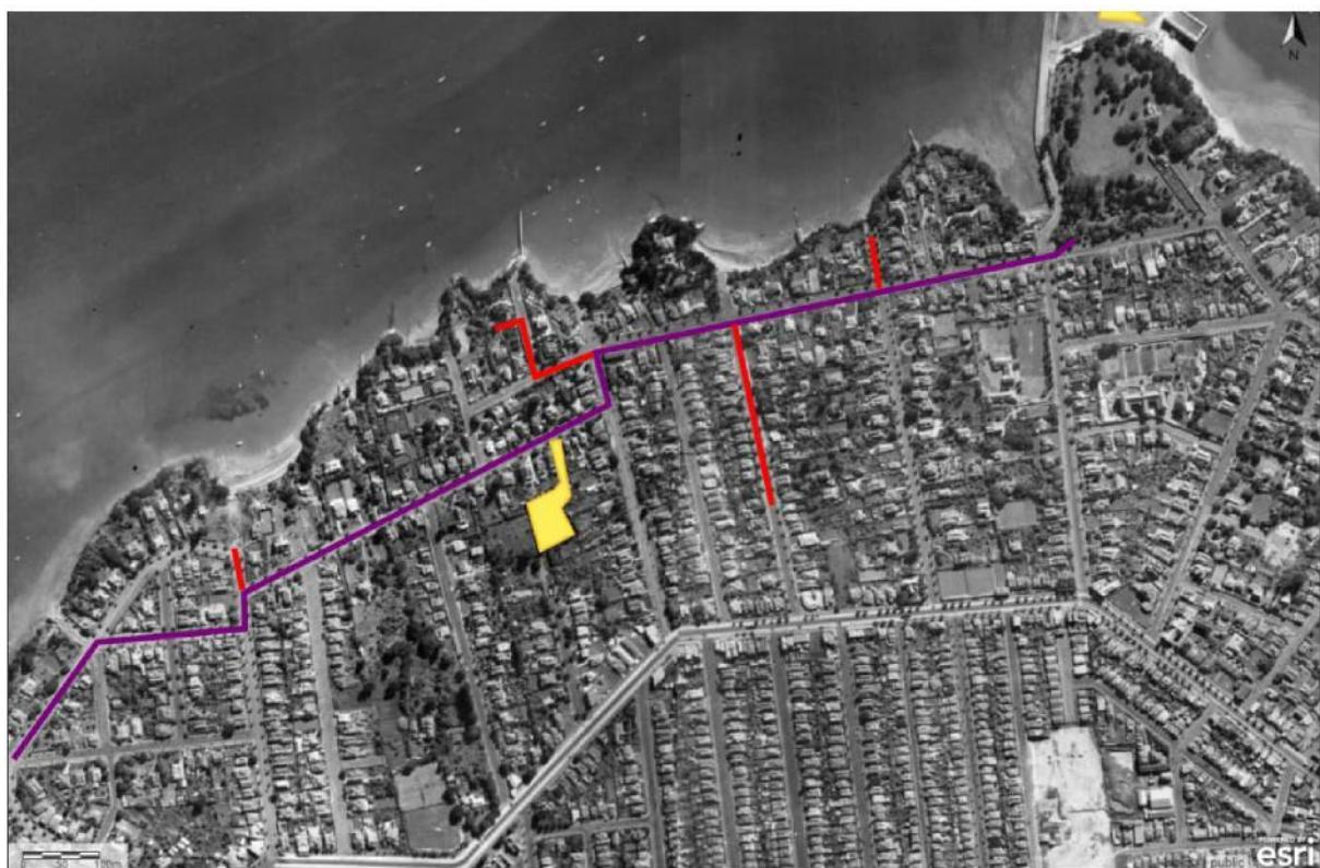
Figure 3.1: 1940 Aerial Photograph, Herne Bay alignment shown in purple, connecting pipes to EOPs in red CSA1 and CSA2 Option 1 highlighted in yellow (Source: Auckland Council Geomaps).
