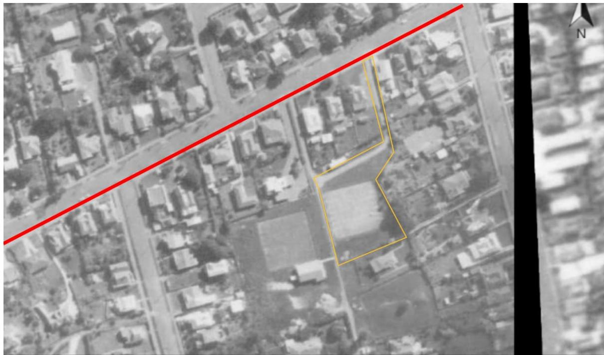
Photograph Appendix B.14: 1959 Aerial photograph with adjacent tunnel allignment in red and CSA1 outlined in yellow (Source: Auckland Council)
