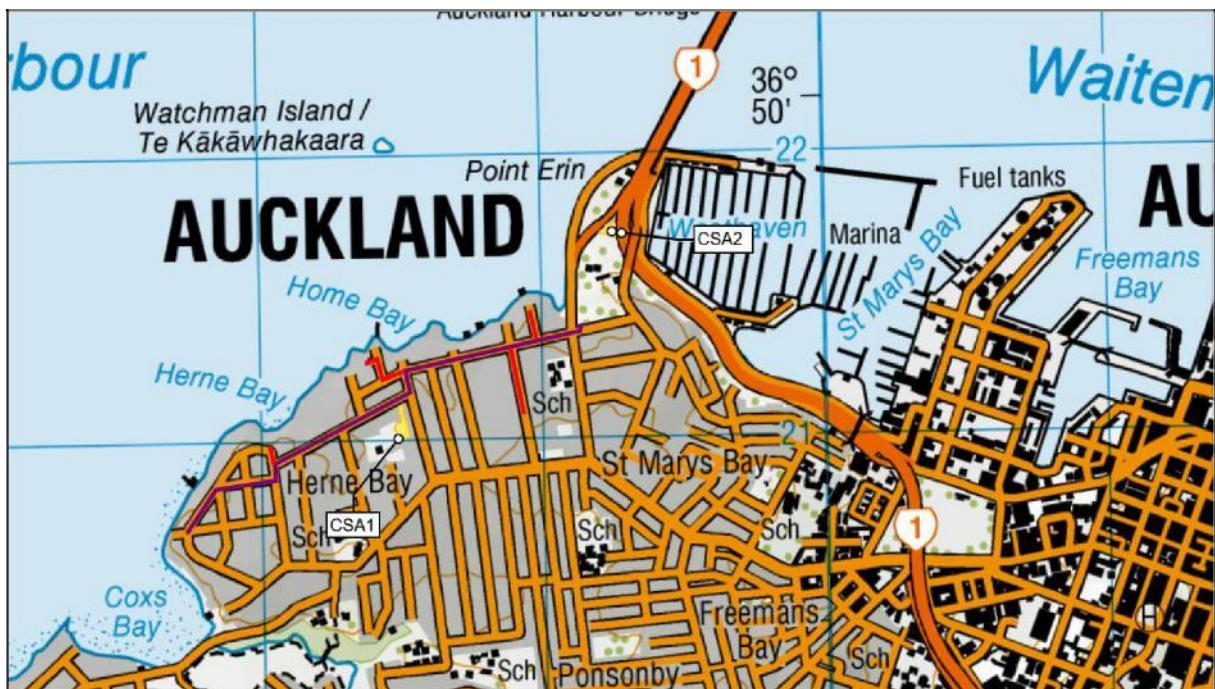
Figure 1.1: Approximate Herne Bay Tunnel alignment shown in purple, connecting pipes to engineered overflow points in red and construction support areas shown in yellow (Source: Topomaps NZ)
