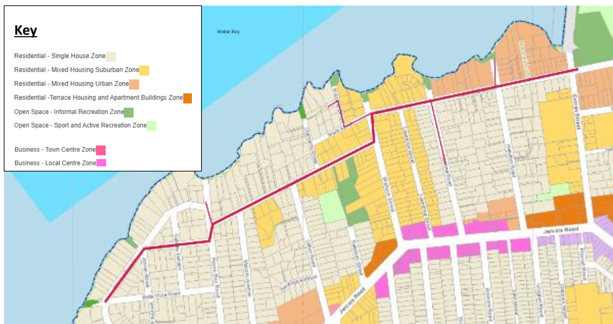
Figure 2.2: Alignment of the trunk sewer line (red line) with the underlying zoning
