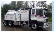
Figure 1 Vacuum truck or hand digging to identify and avoid underground services
