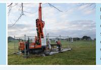
Figure 2 Drilling rig used to collect core samples. The rig may be supported by a four-wheel drive ute and a truck with a water bowser covering an area of approximately 15m<sup>2</sup>
