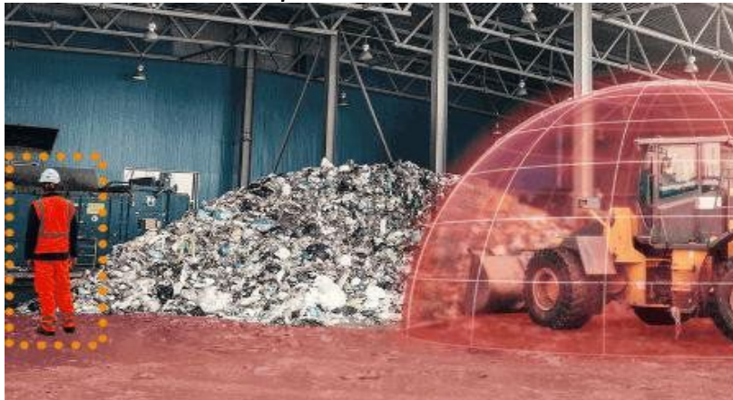
Sensor zone around mobile plant
