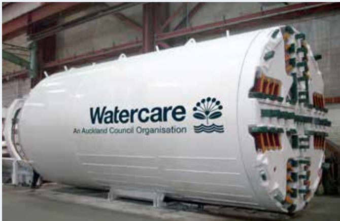
Tunnel boring machine used to build the Hobson Bay tunnel.
