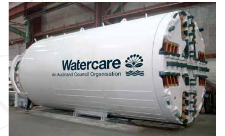
An example of a large tunnel boring machine used for tunnelling deep underground
