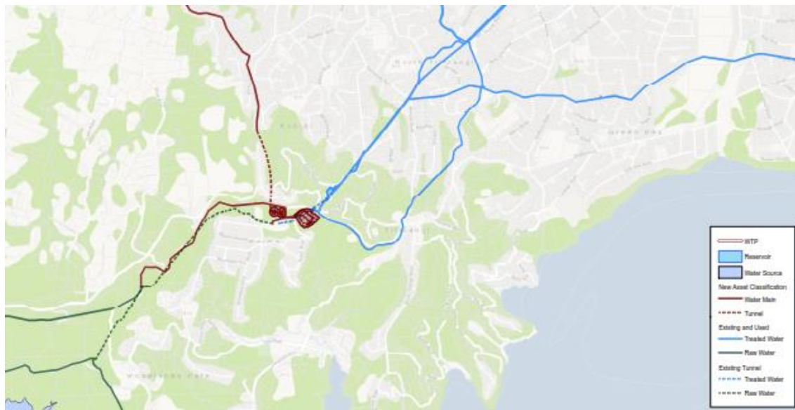
Figure 2.3: Huia WTP Upgrade: Manuka Site Infrastructure Requirements. CH2M Beca drawing no. GIS-6511164-090-01-02D dated March 2017.
