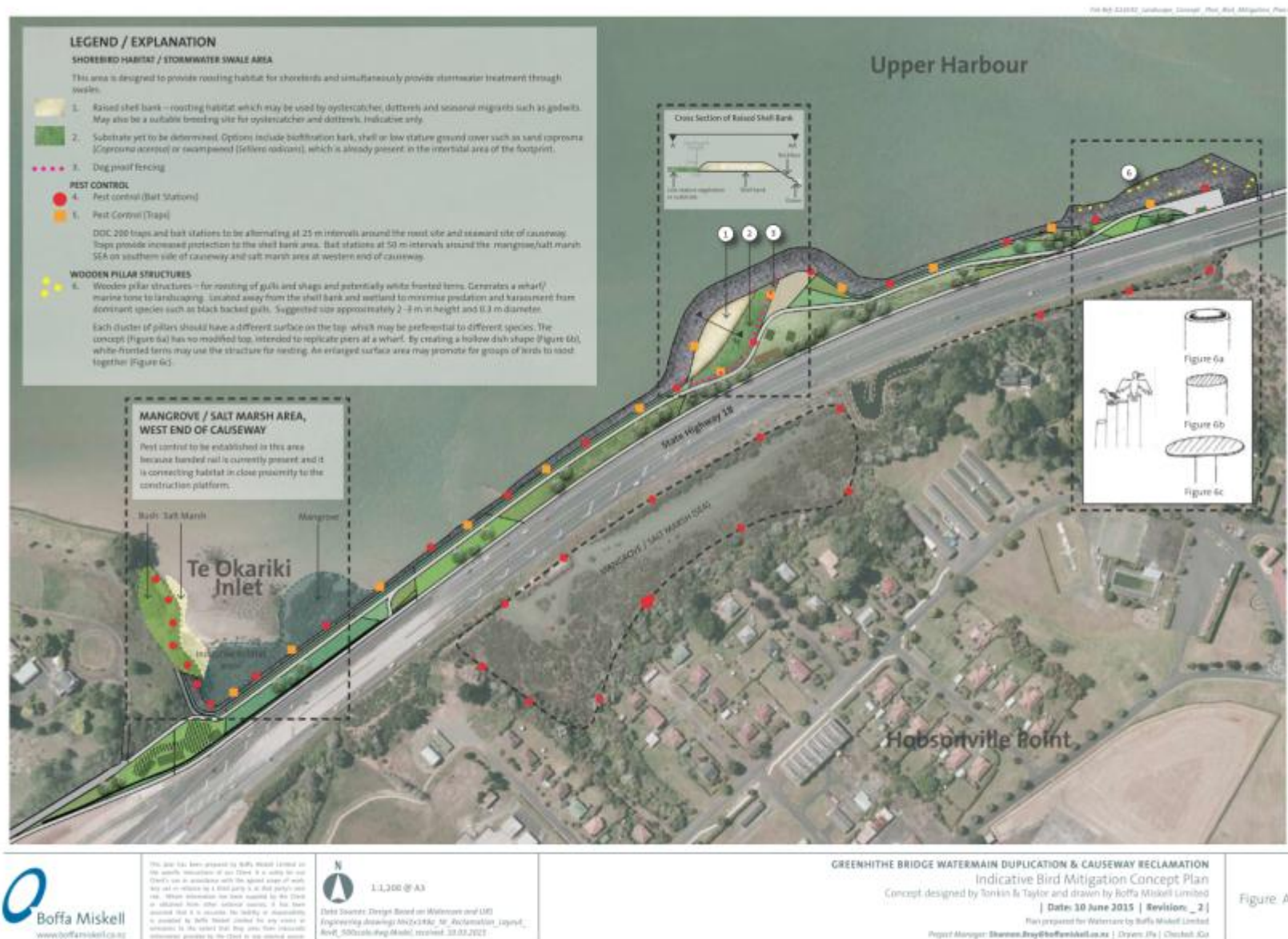
Figure 6-6: GBWD and Causeway Indicative Bird Mitigation Concept Plan
