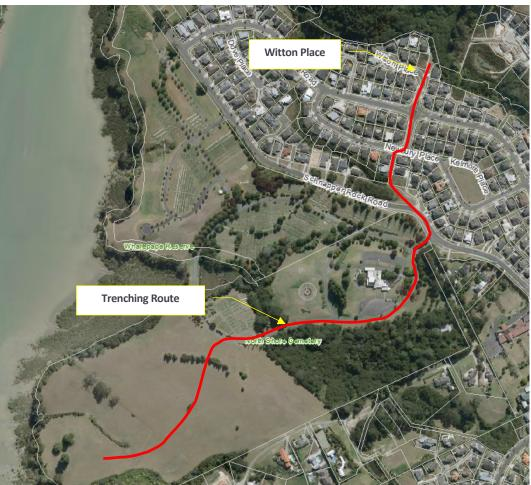
Figure 10: Trenching route through NSMP and adjacent residential
