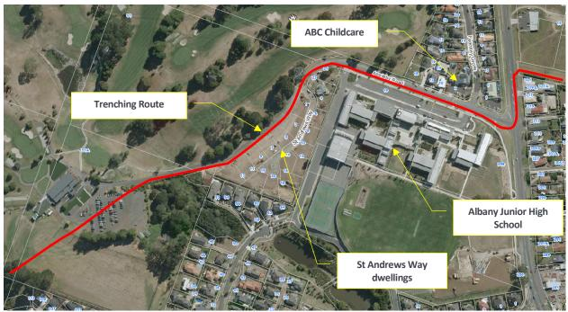
Figure 12: Open cut trenching route and adjacent receivers
