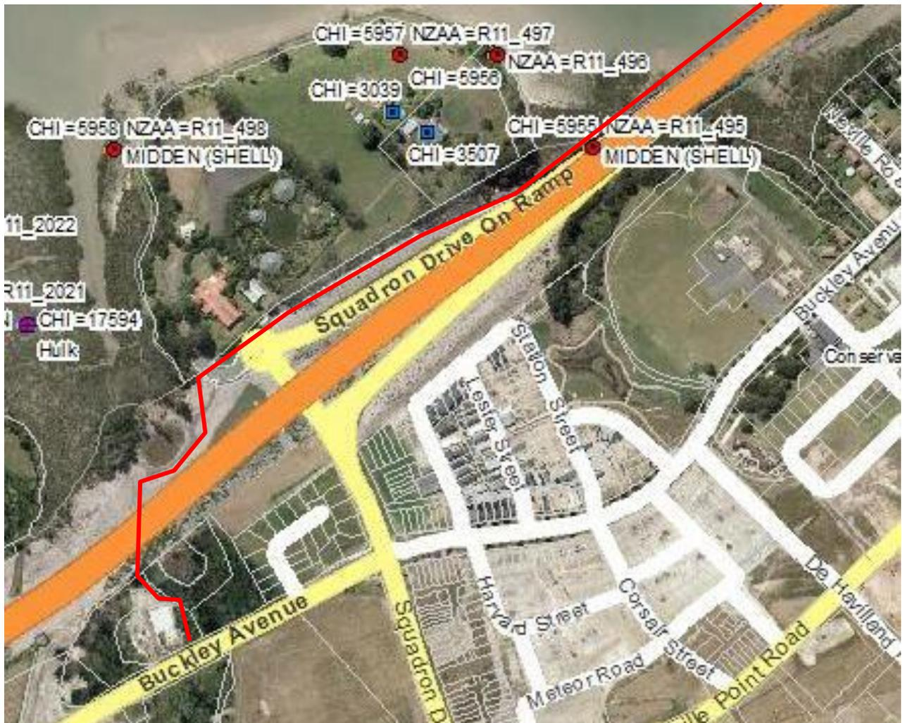
Figure 14. Northern Interceptor Phase 1 alignment (overlaid in red) at Hobsonville, showing distribution of recorded archaeological and historic heritage sites within the general vicinity. Note: site locations are only accurate to within c.100m. Aerial source: Auckland Council GIS 2014
