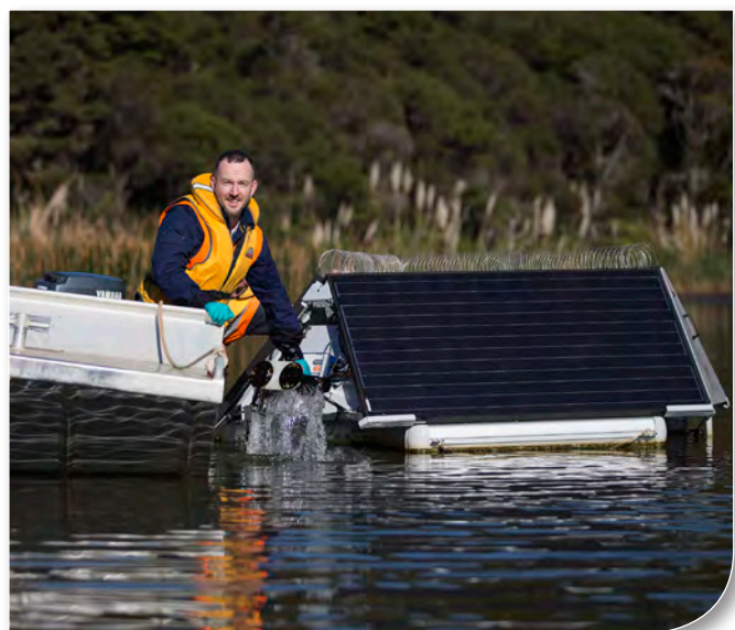
Our headworks team is trialling some new Dutch ultrasonic technology to monitor and combat blue/green algae in the Lower Nihotupu Dam, in the Waitakere Ranges.
